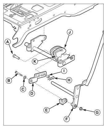
Figure 3. Lift Components - Mowing
